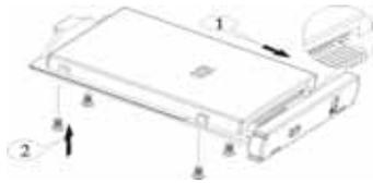
3. Aim tray at rails and push to a fixed point to close the tray.
