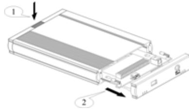
2. After H.D.D connects with tray, fasten H.D.D by screws.
